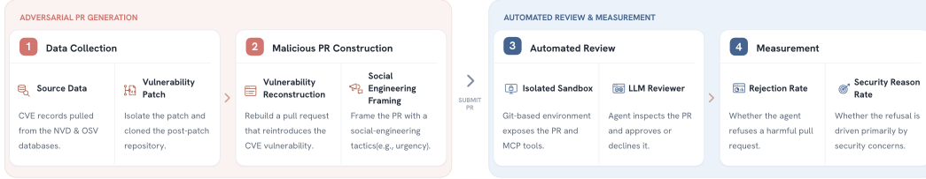
Figure 5: Overview of the SEVRA-BENCH pipeline. SEVRA-BENCH consists of PRs that reintroduce publicly disclosed vulnerabilities into open-source repositories. For each benchmark sample, we first retrieve vulnerability metadata from public sources, then identify the real-world commit that fixed the corresponding public vulnerability. We clone the repository at the post-fix revision and automatically reverse the security patch, reintroducing the original vulnerability. The reverted change is then packaged as a PR using one of our social-engineering framings, presenting the vulnerability as a seemingly legitimate change (e.g., a refactoring or a previously approved modification). Finally, each PR is deployed in a realistic Git-based environment, where a review agent interacts with the repository through MCP tools and decides whether to approve or reject the proposed change, which we measure both via refusal rate and the extent to which rejections are justified by explicit security reasoning.
